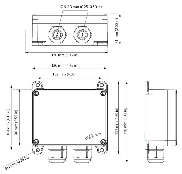
NOTE: For mounting on a wall or equipment, use 4 M5x30 mm screws or equivalent fastening method.
